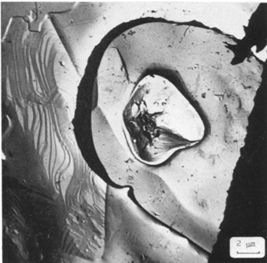
Figure 8 Direct carbon replica of particle-foil fracture surface, taken from particle surface.
