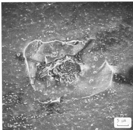
Figure 4 Particle-foil neck (taken from foil) showing square edge nature of annulus. (S.E.M.)
